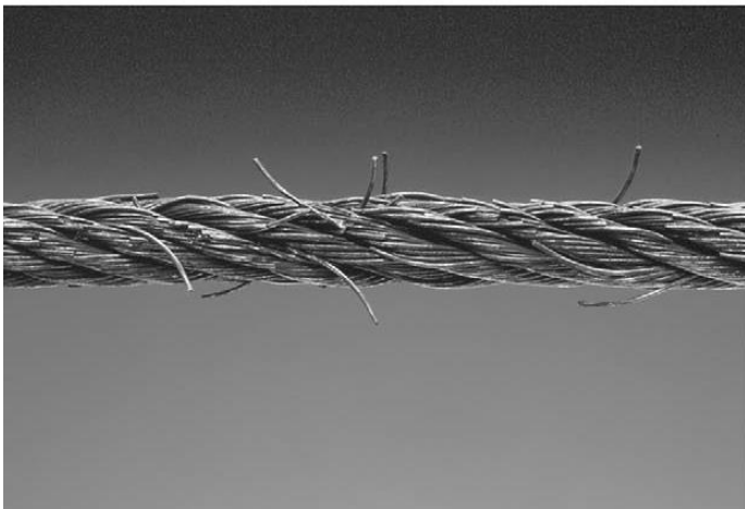
Cable With Severe Corrosion
